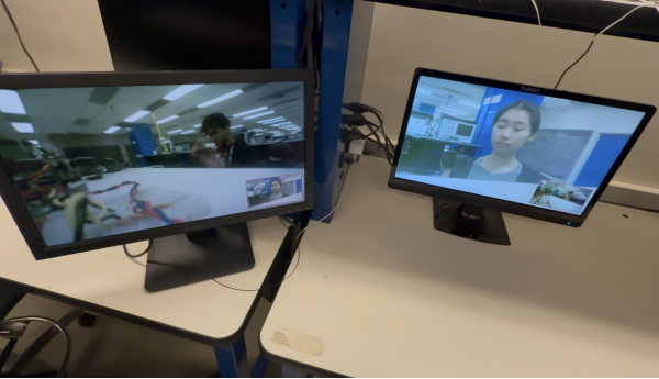
Fig. 1: Working FPGAceTime. Two FPGAs are connected via PMOD B cables, with HDMI outputs displaying remote video feeds and local selfie overlays in the bottom right corners on two monitors.
