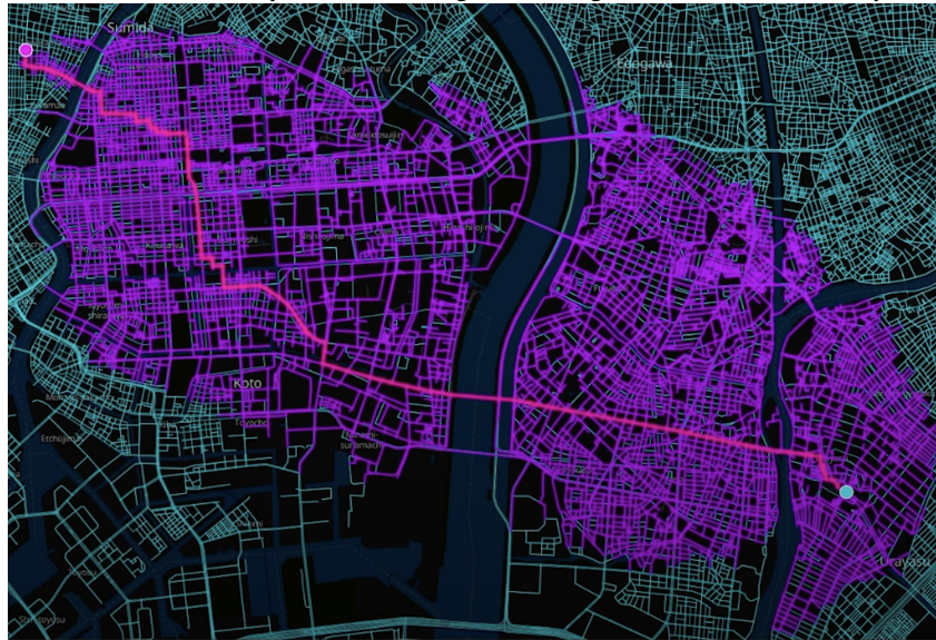
(b) Standard A* uses a heuristic to guide its search from the start node, reducing nodes explored compared to Dijkstra but still visiting irrelevant paths.
