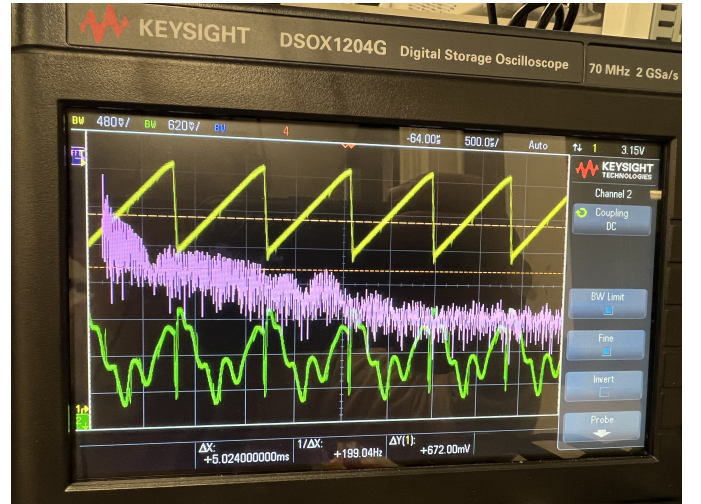
Fig. 4. Oscilloscope capture of the sawtooth wave used to produce frequency chirps (shown in yellow), the baseband signal (shown in green), and its 1-D FFT (shown in purple)
