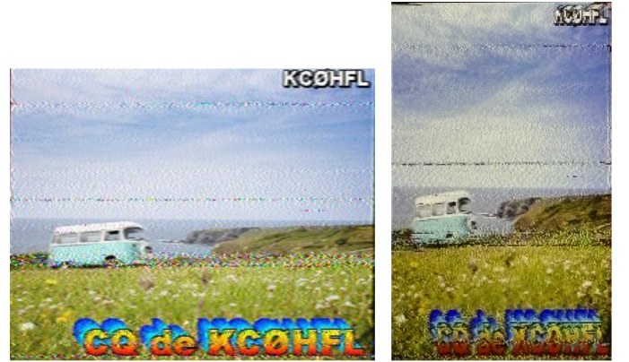
Fig. 10. The left image is the real signal decoded by MMSSTV, while the right is decoded with our receiver. The right image was the output on a monitor captured by a phone.
