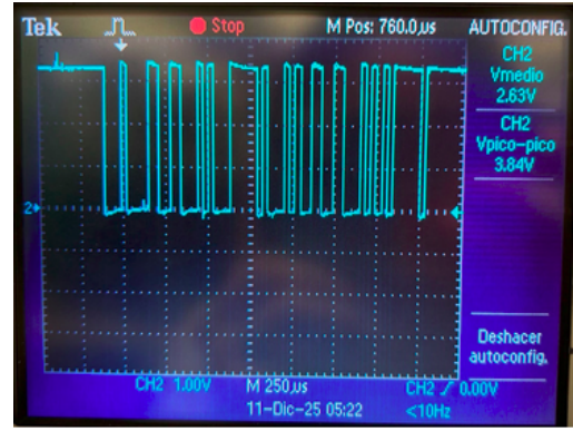
Fig. 9. Scope shot of the MIDI packets sent over UART
