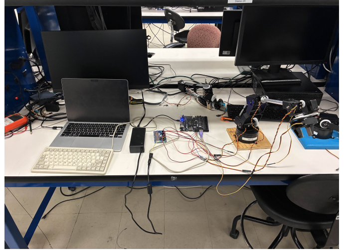
Fig. 1. The physical construction of the FPGArm system. From left to right are the Cherry PS/2 keyboard, generic power supply, Adafruit Servo Shield, AMD Spartan 7 FPGA, and Lynxmotion SES-V1 five-axis robotic arm.
