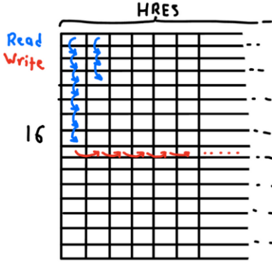
Fig. 3: Read-write logic of the transform buffer
