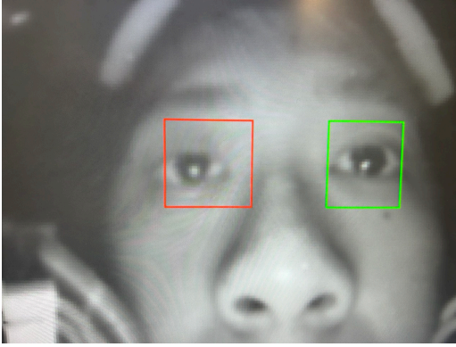
Fig. 5. Partial image of the camera output with eye bounding-boxes overlaid. Notice the bright spot in the middle of the eye as a result of the eye reflecting light from the LED strip within the helmet.
