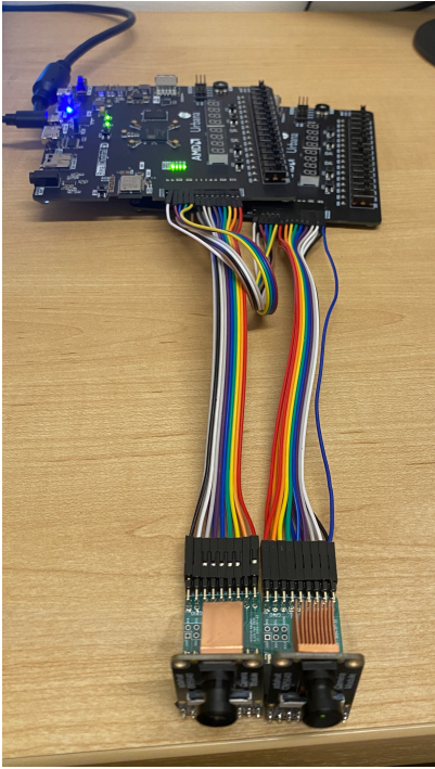
Fig. 3. FPGA setup and PMOD wiring between boards
