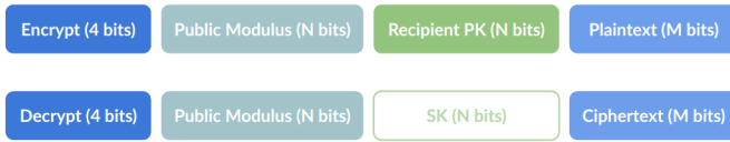
Fig. 3. Communication packet structure. The deserializer must pull the user’s secret key from BRAM when it is in decrypt mode.
