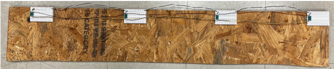
Fig. 1: Physical design of the linear microphone array
