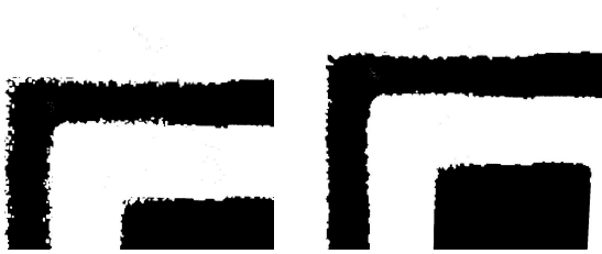
Figure 1. Image on the left: Before applying the denoising convolution kernel. Image on the right: After applying the denoising convolution kernel.
