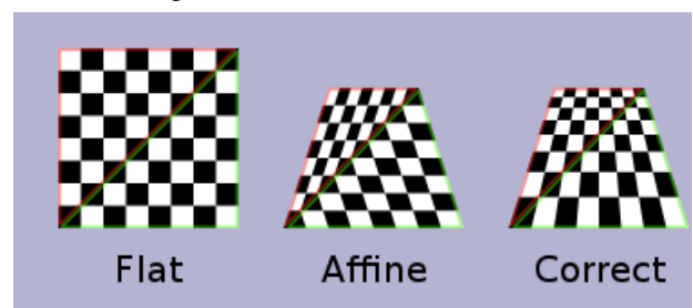
Fig. 9. Screen space (Affine) interpolation of UVs vs perspective correct interpolation. Ours and the PS1 would look like the Affine one.
