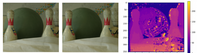
Fig. 2. Left: left camera view, Center: right camera view, Right: disparity map from SSD
