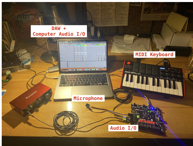
Fig. 1: Full vocoder system with typical audio production usecase
