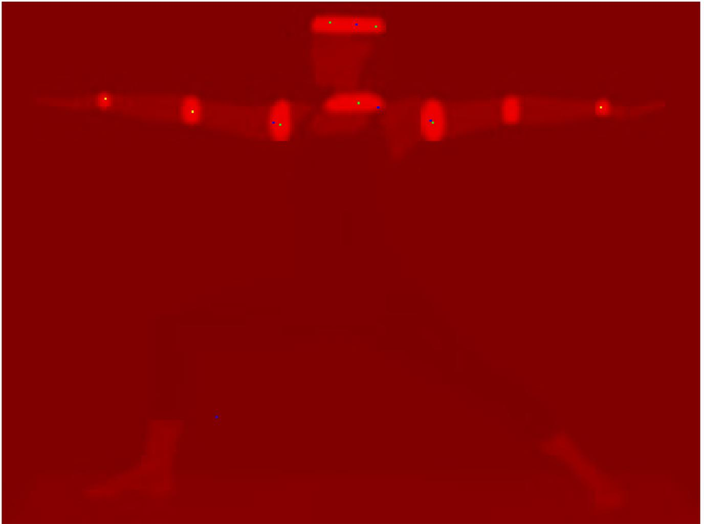
Fig. 6: Seed 1 chroma red image with visualized centroids. Color scheme: green pixels depict centroids determined by scikit-learn's machine learning package for k-means clustering, blue pixels depict centroids determined by our Verilog algorithm, yellow pixels depict centroids identified by both.
