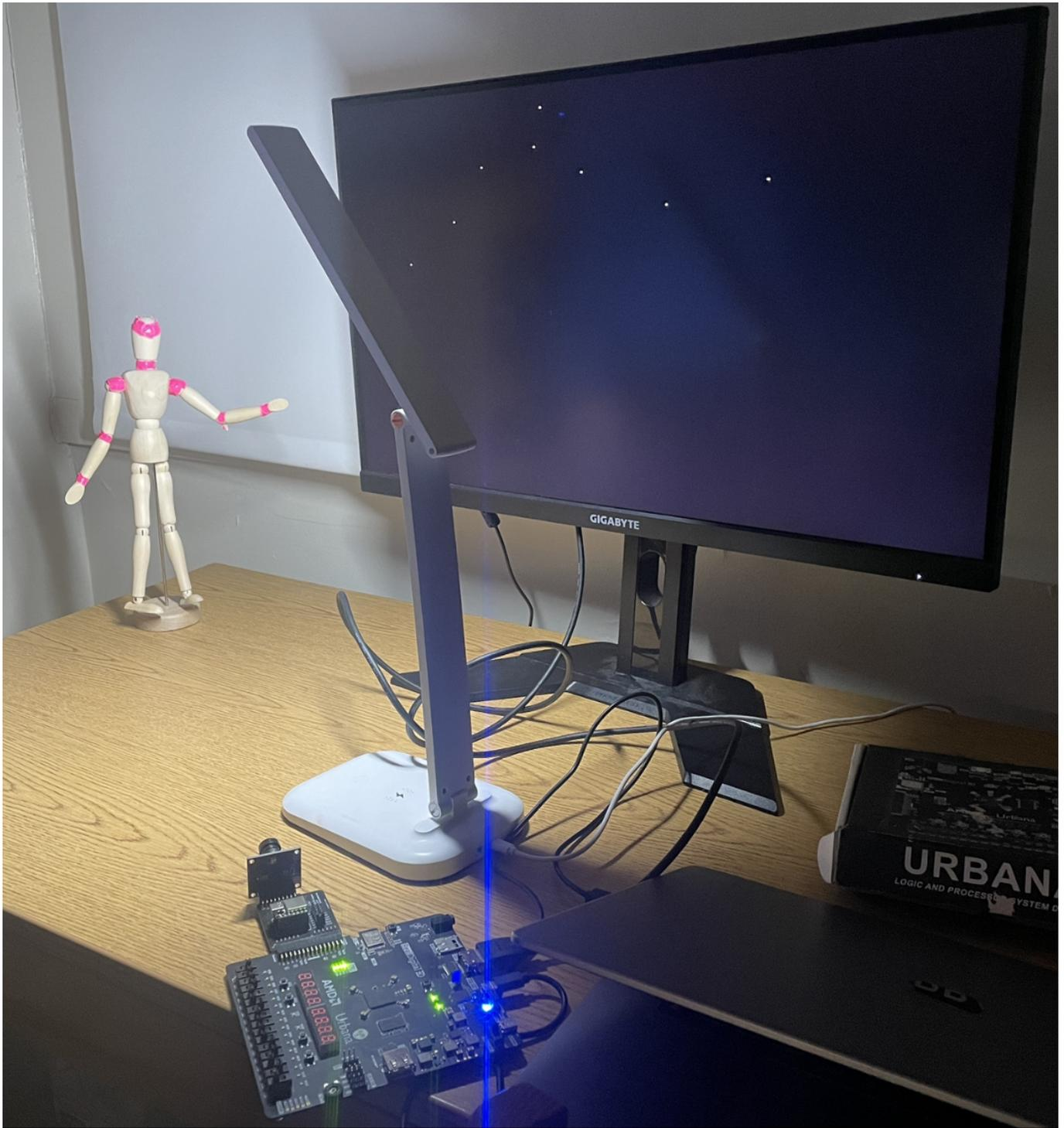
Fig. 11: Centroids displayed, roughly representing the doll's pose
