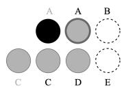
When the line buffer has sent along these two new values, the "old **B**" becomes the "new **A**" to be dithered, "old **D**" becomes "new **C**", and "old **E**" becomes "new **D**". In the diagram below, all pixels shaded in with grey are now updated values that do not match what came out of the camera/SD Card and was written into the line buffer.
