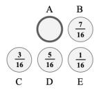
When the dithering of  $\mathbf{A}$  is complete, pixels  $\mathbf{B}$  through  $\mathbf{E}$  will take on a new value equal to their previous value plus the quantization error scaled by the fraction they are labeled with above.
