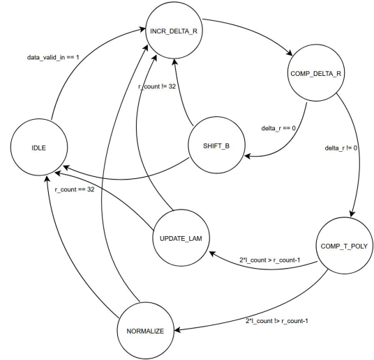
Fig. 6. Finite State Machine of the Berlekamp-Massey algorithm.
