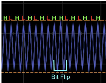
Fig. 4 – Observed receive signal with highlighted bit flip
