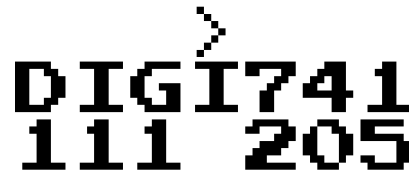
Fig. 8. An example sprite for a plane with the call sign “DIGI741” that is moving at 111 degrees at a speed of 205 knots
