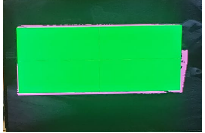
Fig. 4. Bounding Box algorithm generating a green rectangle encompassing the pink plastic object
