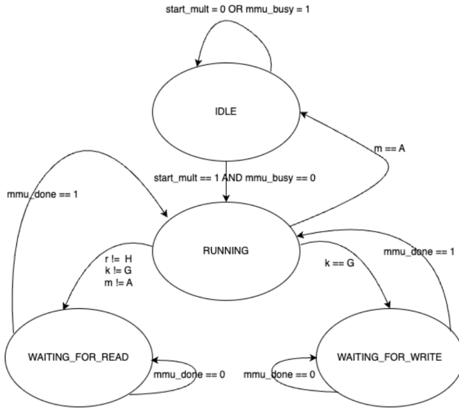
Extra Fig 3: Memory Management Unit State Diagram
