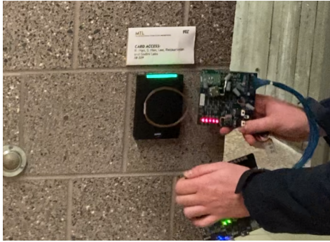
Fig. 13. Our PICC, emulating Matthew's MIT ID, successfully opens the door of a lab that Matthew has access to.
