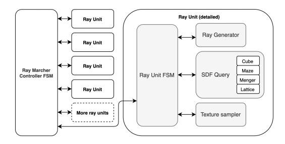
Fig. 4. Block diagram for the Ray Marcher
