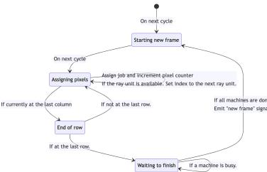
Fig. 3. State diagram for the Ray Marcher Controller
