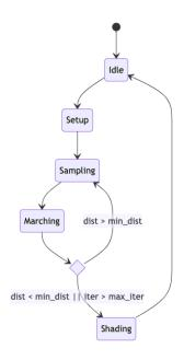
Fig. 6. State diagram for the Ray Unit
