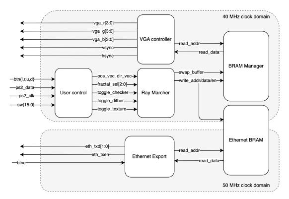
Fig. 1. Block diagram for the top level of the system
