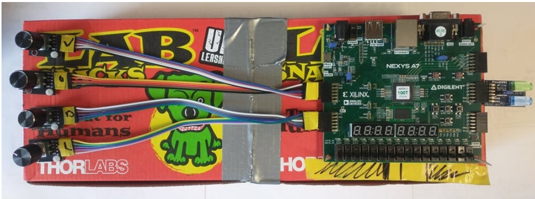
Figure 1: The main hardware setup. The four rotary encoders are connected to the left of the Nexys board, while the Pmod I2S2 can be seen on the right.
