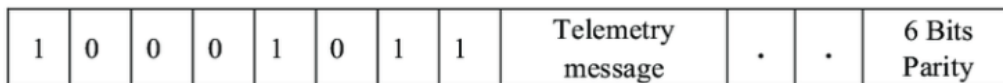
Fig8. Structure of NAV Message Word 1, which includes the preamble. This is transmitted at the start of every subframe (every 6s)
