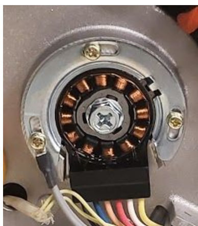
Left : the backside of the motor, with the variable reluctance resolver shown
