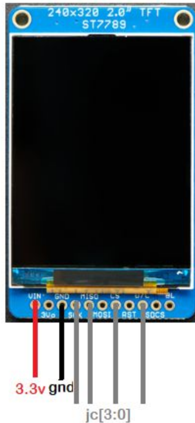
Figure 7: Wiring diagram for the displays. The data ports are connected to jc in the order they are on the display PCB, with SCK connected to jc[3] and D/C connected to jc[0]
