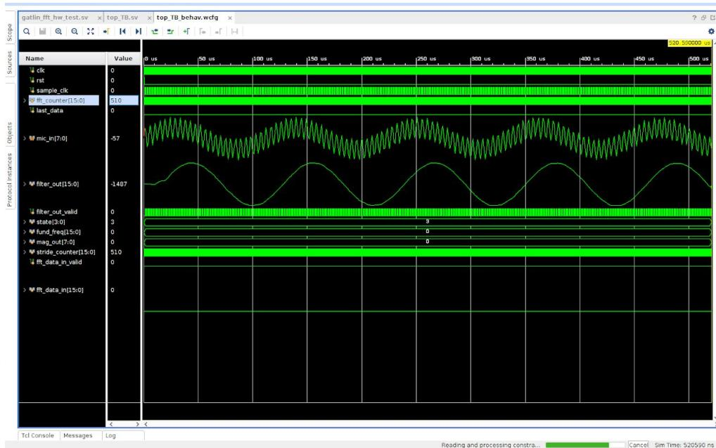
The filter very effectively filters out the higher frequency.
