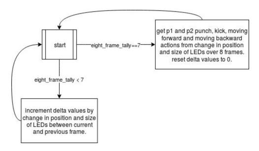
Get actions FSM: Calculates the change in location of the LEDs in the x and y direction and the change in size of the LEDs. On the eighth frame (when eight\_frame\_tally==7), uses those to determine which action the LED is making and set the boolean variables p1\_punch, p1\_kick, p1\_moving\_forward, p1\_moving\_backward, p2\_punch, p2\_kick, p2\_moving\_forward, and p2\_moving\_backward.
