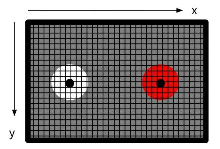
The rate of change of these coordinates over a set of 8 consecutive frames is used to calculate the average rate of change of the players' hands in the x and y directions, as well as the rate of change in the size of the players' LEDs. The magnitude and sign of the rates of changes are stored separately. This information is used to classify the hand gesture as one of the following states: none, punching, kicking, moving forwards, and moving backwards.
