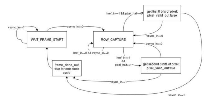
Camera FSM: Gets the pixels from the camera and outputs when the pixel output is valid and when the frame is done.
