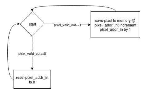
Memory FSM: When the pixel output of the camera module is valid, stores it in memory at the correct address.
