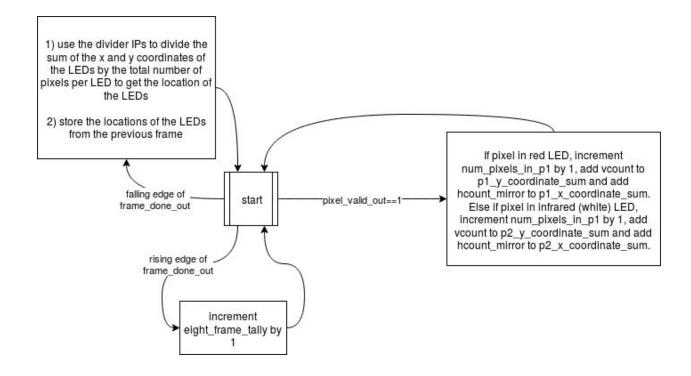
Extract location of LEDs FSM: When the pixel output of the camera module is valid, updates the number of pixels from each LED and the sum of their x and y coordinates. On the falling edge of frame\_done\_out uses those values to calculate the locations of the LEDs in the frame and store the previous locations of the LEDs in variables. Also increments eight\_frame\_tally on the rising edge of frame\_done\_out.
