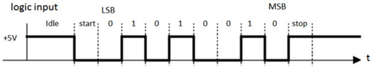
Figure 2: Waveform for one byte's transmission
