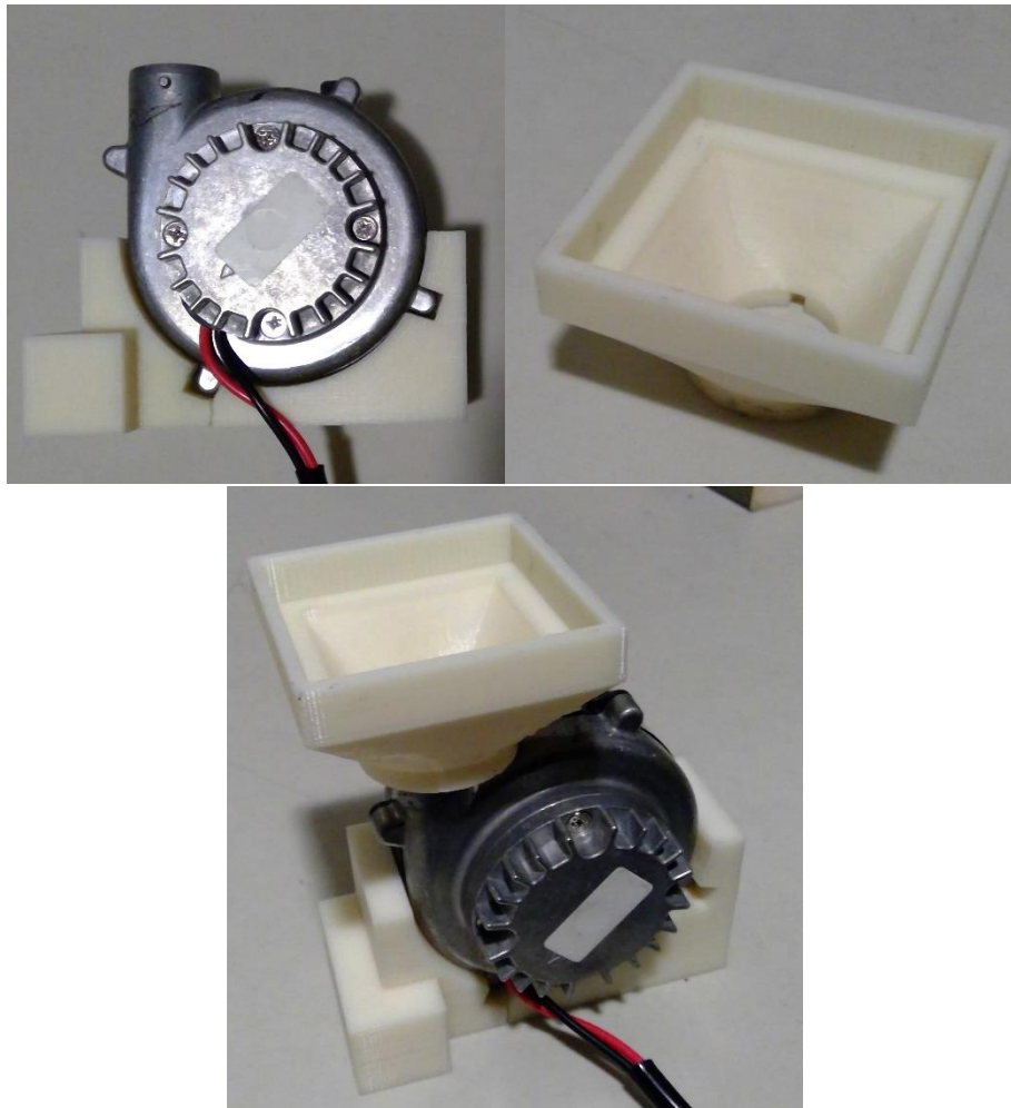
Figure X: The fan slotted into the base part, the fan's connection to the tower, and the fan assembled with both pieces.
