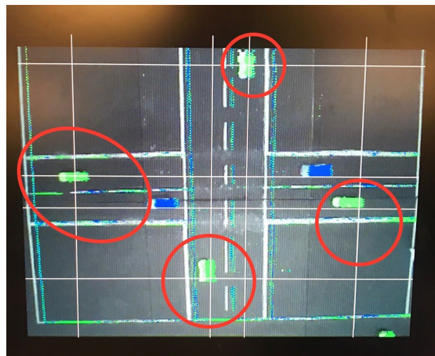
Figure 4: Illustration of cross hairs detecting cars
