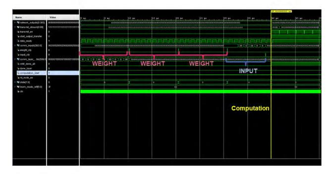
Depiction in simulation of the entire process from the simulated transmission of weights and inputs, computation of outputs, and transmission of these outputs.
