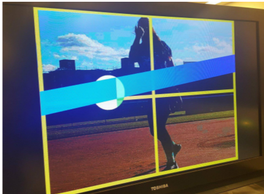
Figure 5. Graphical display with picture in background, strikezone outlined in yellow, blue angled bat, and ball indicating point of contact and hit timing
