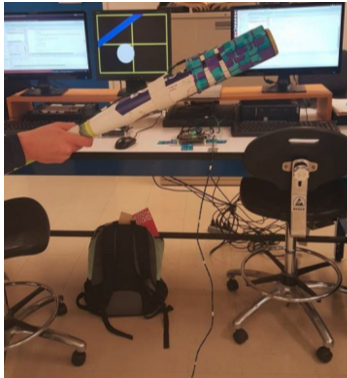
Figure 12. Bat angle displayed in real-time for testing. Also notice the earlier prototype version, with a long connected wire and IMU sensors attached at the end of the bat
