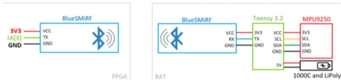
Figure 4. Communication system high level diagram. The bluetooth modules were originally replaced with a long wire between Teensy TX pin and FPGA JA[3].
