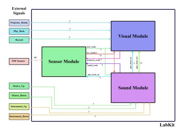
Testing the visual module will involve both writing test jigs and conducting physical tests. Since there is a lot of imagery involved, physical tests will involve examining the piano images to make sure they look correct and to see if there is noticeable delay in image changes after key presses, and measuring projected image sizes to see if they match our expected dimensions. Test jigs will test that all internal signals are getting sent at the correct clock edges.
