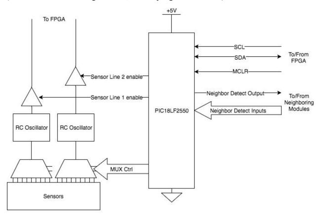
Each block will have 4 connectors on each edge. These connectors will be used to connect adjacent blocks as well as to the FPGA. Each connector will have the following I/O pins:
