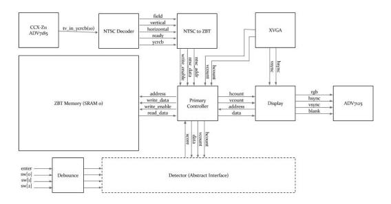
Note that the detector module in the above block diagram - see dashed lines - is an abstract interface which ingests pixel data and button presses and returns scores for each location in the frame. The key responsibility of this component is to recognize and track objects, and we propose 2 different concrete implementations based on traditional and modern computer vision techniques, respectively.
