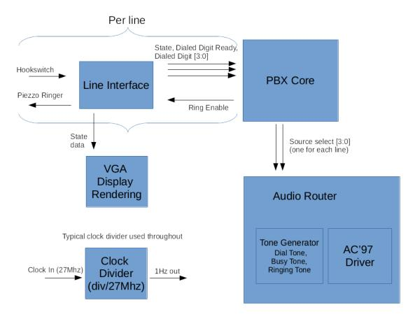
Each extension/line has a *line\_interface* module that performs the low-level phone interfacing. By monitoring the hookswitch input from the interface circuitry (see next section), this module's state machine outputs decoded dialed digits and a "phone active" signal when picked up. It also includes a siren tone generator for driving a piezo ringer at the standard North American ring cadence of 2 seconds on, 4 seconds off.
