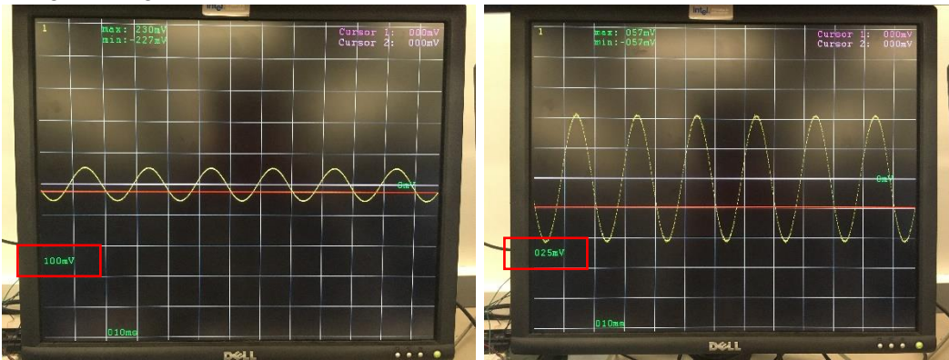
The volts per division is indicated in the red box
