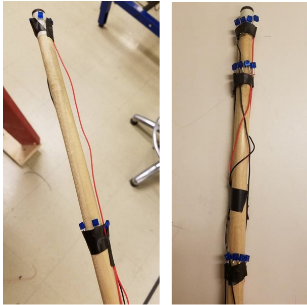
Figure 3.3: (a) First cue LED configuration with evenly spaced diodes. (b) Second cue LED configuration with diodes angled upwards.
