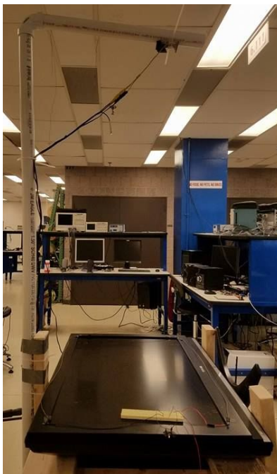
Figure 2.1: Hardware setup with NTSC camera mounted above TV screen.
