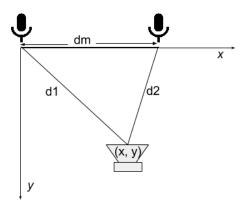
With two distances calculated from the previous module, this module produces the x and y coordinate of the speaker in real-time. This triangulation is requires solving two trigonometric equations which are difficult to perform on FPGA, so we will make a lookup table to map pairs of distances to their respective coordinates.
