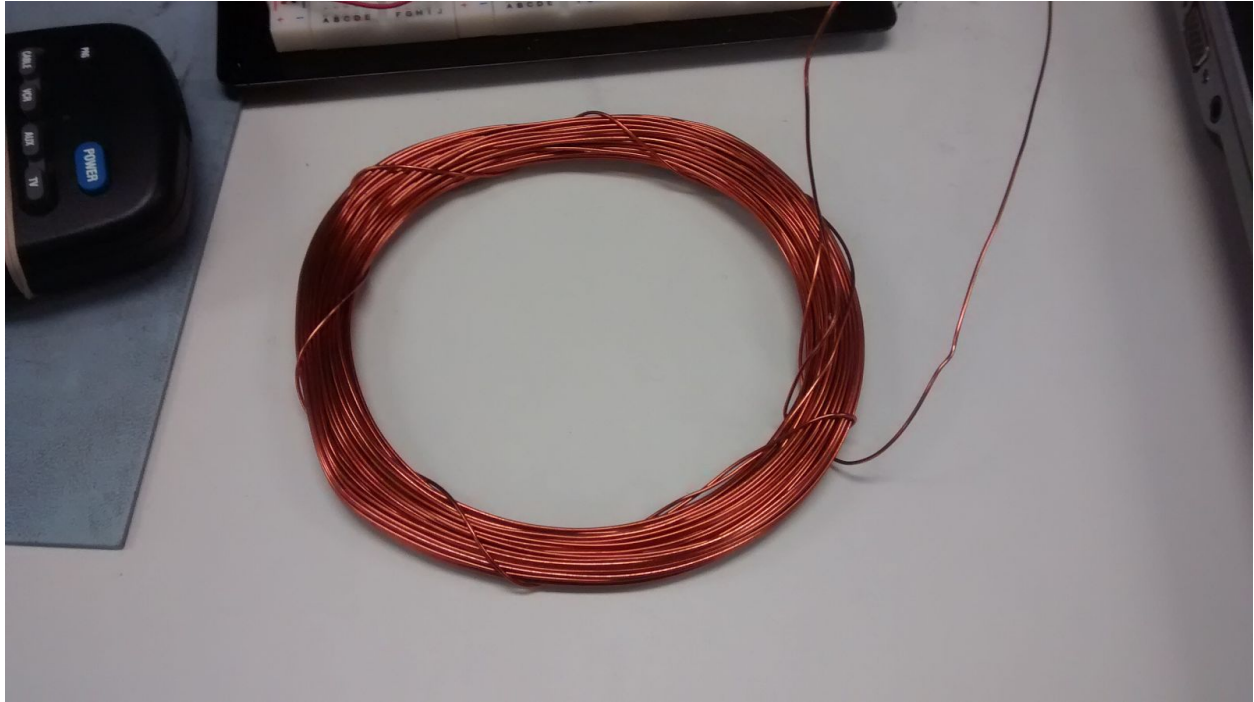
Figure 2: Custom coil used as the antenna
