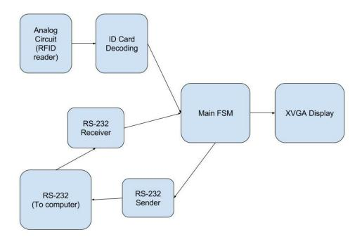
Figure 1: Overall (simplified) Block Diagram
