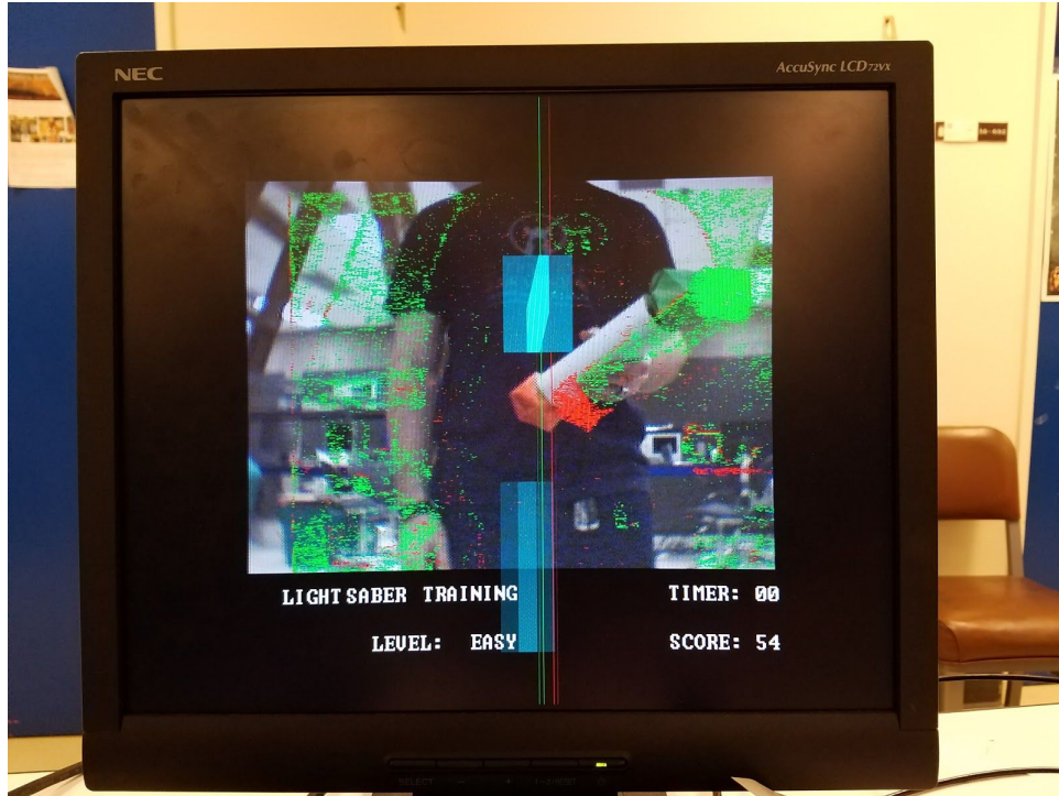
Figure illustrating noise, as well as low levels of saturation. The pixel offset is due to the latency on the dividers.
