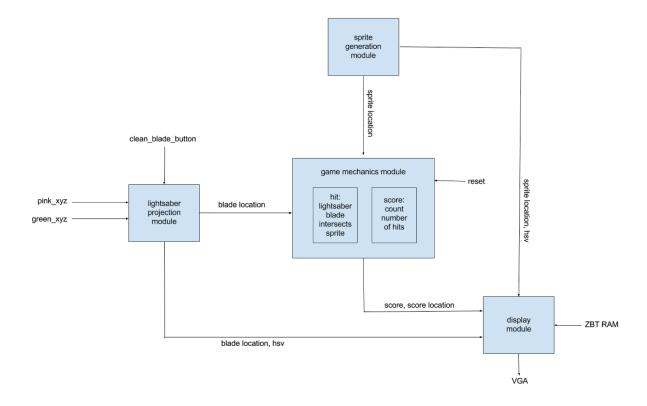
The gameplay component of the project will take the outputs of the sensor and video/image tracking modules to create a projection of the lightsaber blade. Additionally, the sprite generator will create objects on screen that can be hit by the lightsaber, increasing the player's score according to the game logic. The lightsaber blade, sprites, and score will be overlaid onto the video image held in the ZBT RAM.
