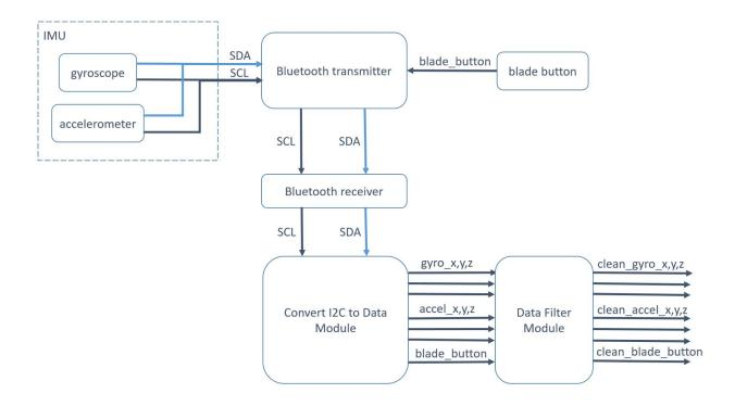
To help determine the location of the lightsaber handle in physical space, we will be putting an IMU on the handle to gather gyroscope and accelerometer data. The handle will also have a button that serves as an input into the game as to when the blade should extend or retract. To allow ease of use and not have wires dangling from the handle, the IMU and blade button data will be transmitted via Bluetooth. The Bluetooth transmitter will receive the IMU data via I2C to transmit.
