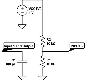
In this circuit we connect the two leads of the 3.5mm jack to input 1 and 2. Input 2's DC bias is suddenly raised to 0.5V. Now input 1, as a result, will have a bias of 0.5V and passes an AC signal. We measure our output from input 1.
