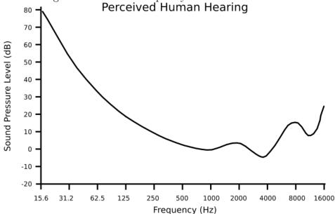
As a result, the following frequencies were used in the final setup: 80Hz, 100Hz, 200Hz, 300Hz, 500Hz, 800Hz, 1000Hz, 1500Hz, 2000Hz, 3000Hz, 5000Hz, 8000Hz. The microphone used had a frequency range from 80Hz to 12,000Hz. Various tones with frequencies up to 15,000Hz were tested, though it was found that it was difficult to perceive sound above 8,000Hz.
