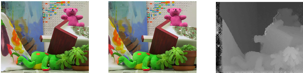
Figure 21: Left image, Right image and computed Depth Map
