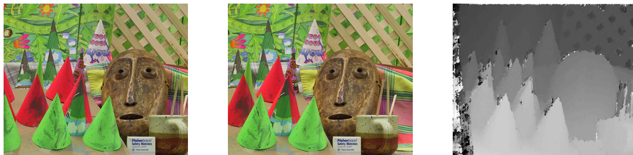
Figure 17: Left image, Right image and computed Depth Map
