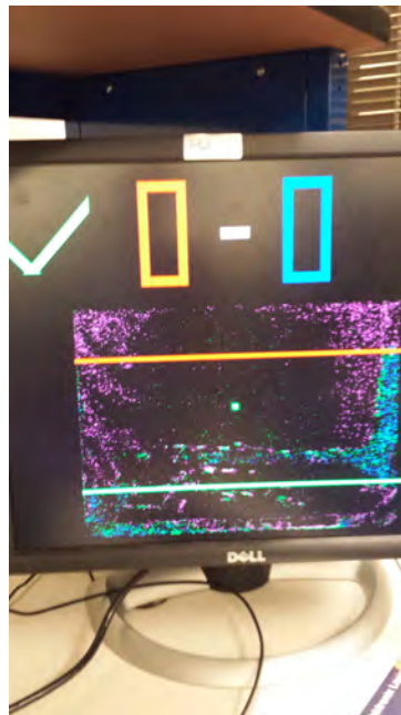
Figure 2.1: VGA Display with blacked out camera image except for pixels matching combinations of HSV.
