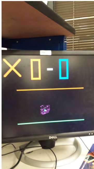
Figure 2.3: VGA Display with blacked out camera image and matched values only around COM point
