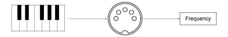
The deserializer module takes input from the keyboard and extracts data on the pitch of the most recent key press.
